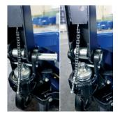
3. Important information regarding the chain assembly: First make sure that the chain is outside the drawbar. Now align the two holes on the tiller and the housing and put the axle bolt through.
