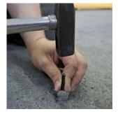
2. Use a hammer to drive in the locking pin on one side and insert the axle bolt into the holder. Make sure that the hole in the axle bolt is facing forward. If the hole is on the other side, insert the axle bolt from the other side.
